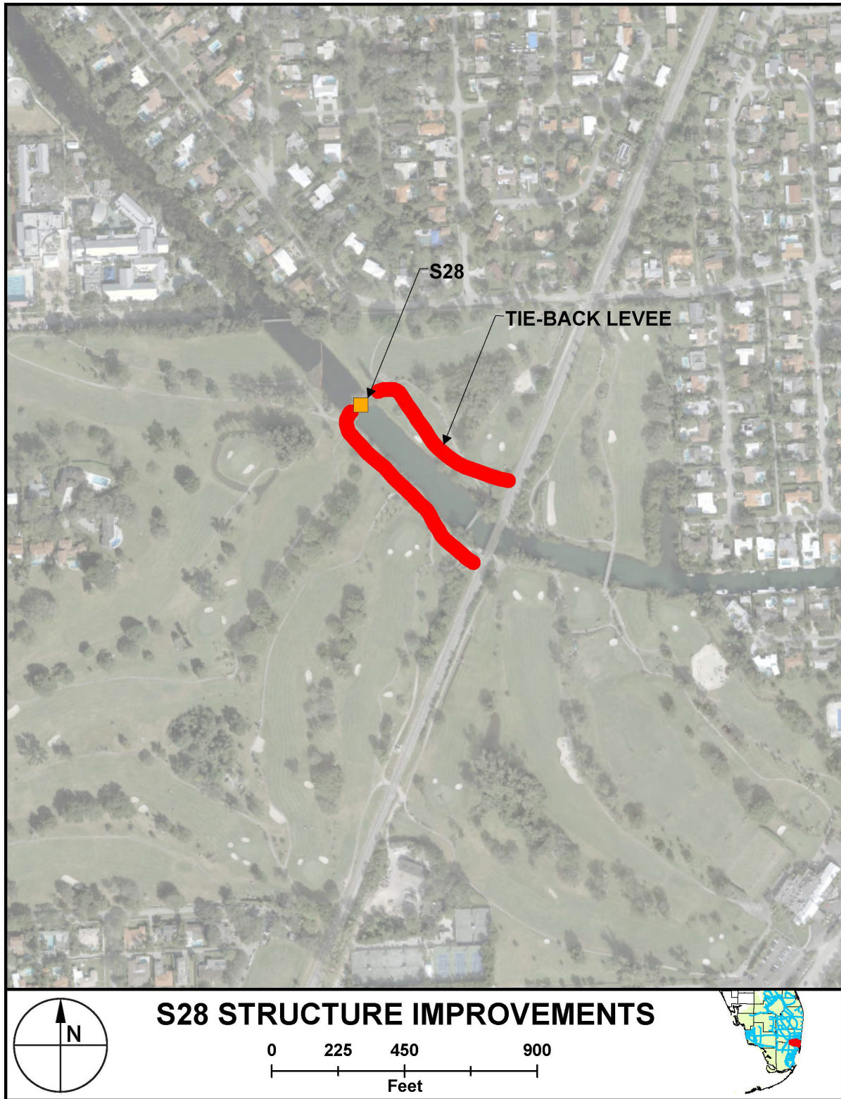
Figure 3.3 Generalized Schematic of Tie-back Levees at S-28
